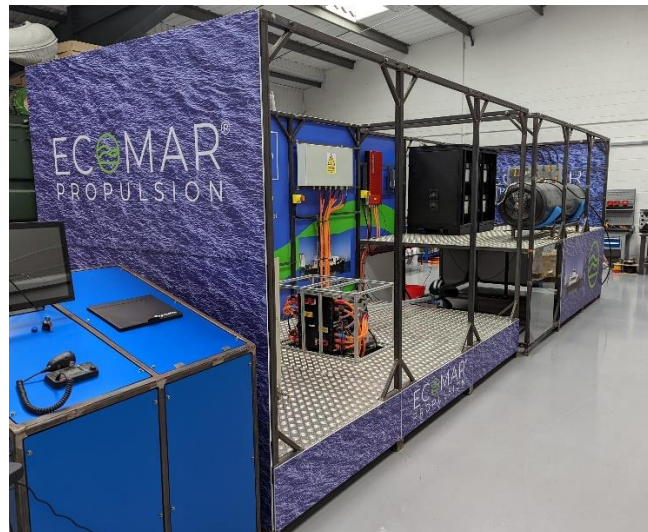
Figure 1 – Ecomar Demonstrator Example, this project aims to demonstrate the engine room of a 44 metre OSE designed Ship for Zero Emission Propulsion (credit: Ecomar)
